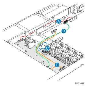
Figure 49. SCSI Cable Routing Through Notches in Metal Air Baffle
